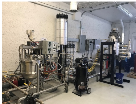
STRATCO® R&D Pilot Unit used for research of industrial processes. Benefits include less raw materials, less production time and increased yields.
