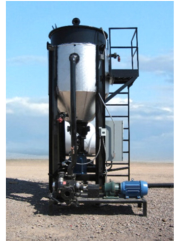
Modified Asphalt Contactor™ reactor used in the Asphalt Shingle Manufacturing process
