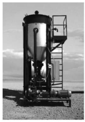
Modified Asphalt Contactor™ reactor used in the Asphalt Shingle Manufacturing process
